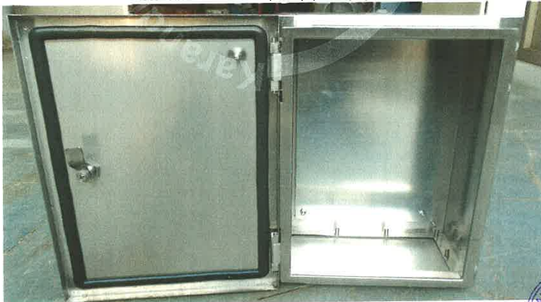
Picture2: No ingress of powder & water observed
